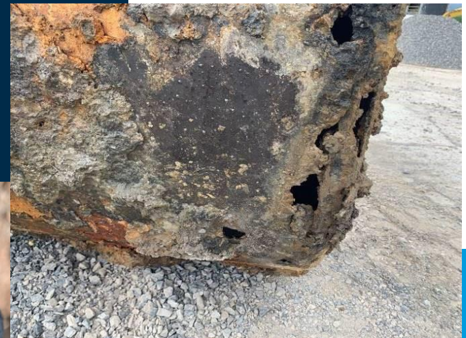
Excavation of 6 Leaking Underground Storage Tanks
